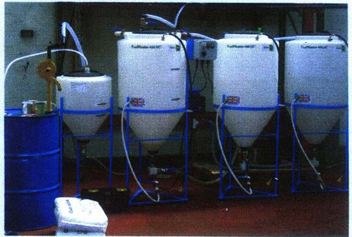
A transesterification system takes waste vegetable oil or rapeseed oil, blending the raw material with methanol and sodium hydroxide before allowing the end product to settle prior to final refining.
