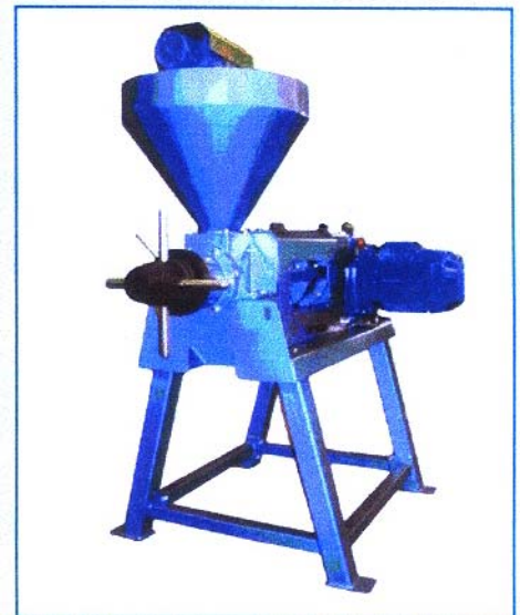
Alvan Blanch has developed its first farm scale oil screw press to crush oilseed rape ready for processing.
