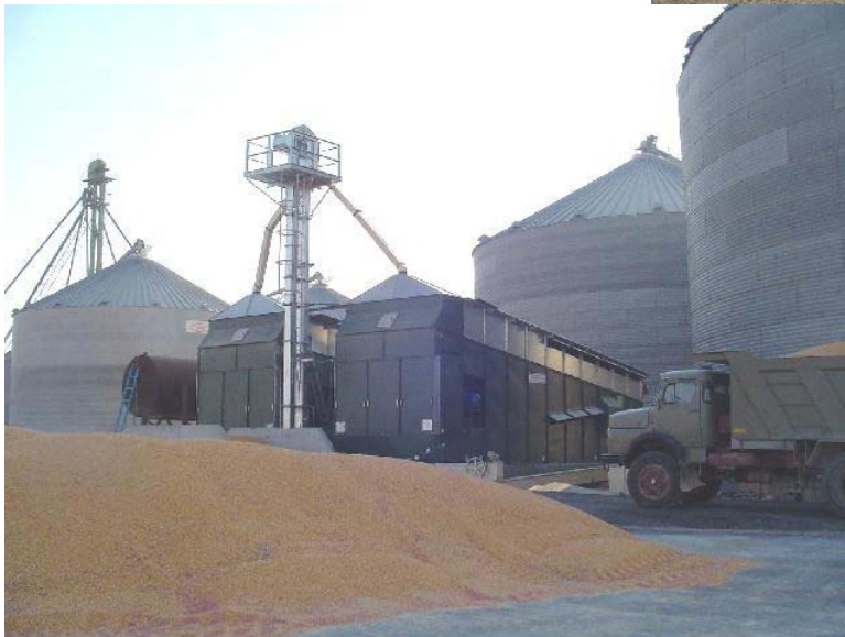
Maize Storage System with twin driers (Saudi Arabia)
