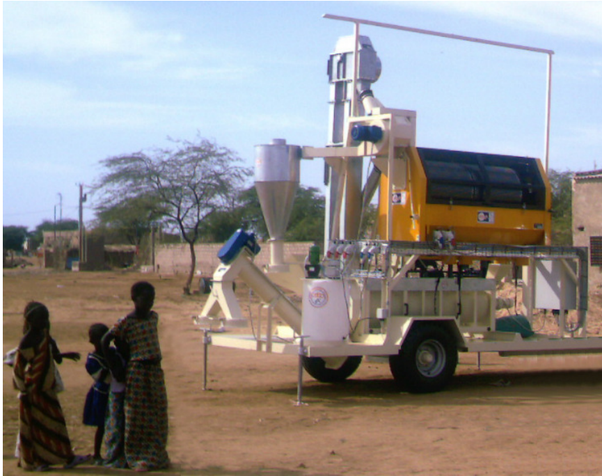
Above Photograph: 1 tonne/ hour rice multiplication system for Senegal.
