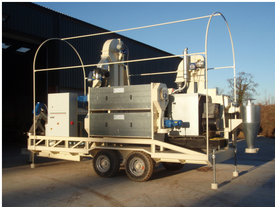
LHS shot: Control panel, indented cylinders and generator set.
