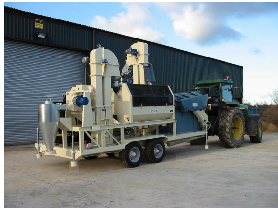
RHS shot: Aspirator and cyclone, elevator, rotary cleaner and gravity separator.
