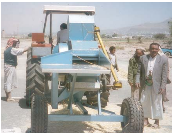
Ease of mobility: Aspra master with Tractor PTO drive - arrives for wheat threshing in Yemen
