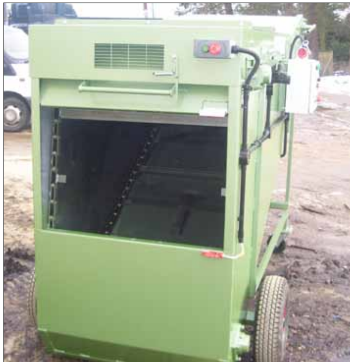
Roller loading door takes baled peat
