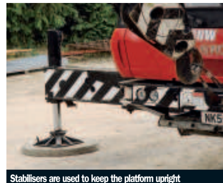
Stabilisers are used to keep the platform upright
