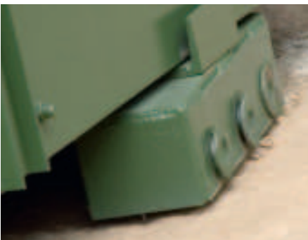
Special rollers are used under the drier
