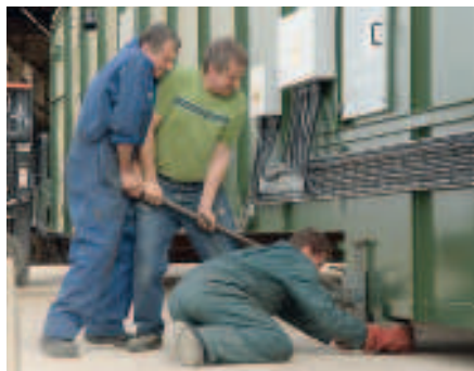
Jacks and lump hammers change the drier's direction
