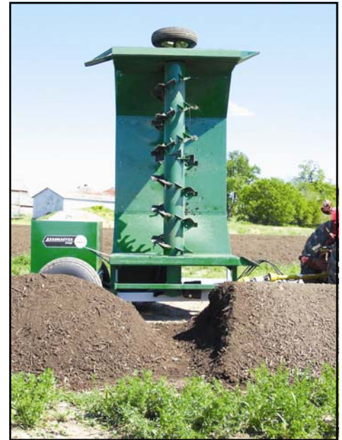
The Aeromaster's drum assembly can be lifted completely out of the windrow.
