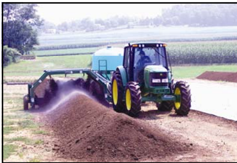
The unique water and inoculation system assures even moisture to every particle as the turner moves through the windrow.
