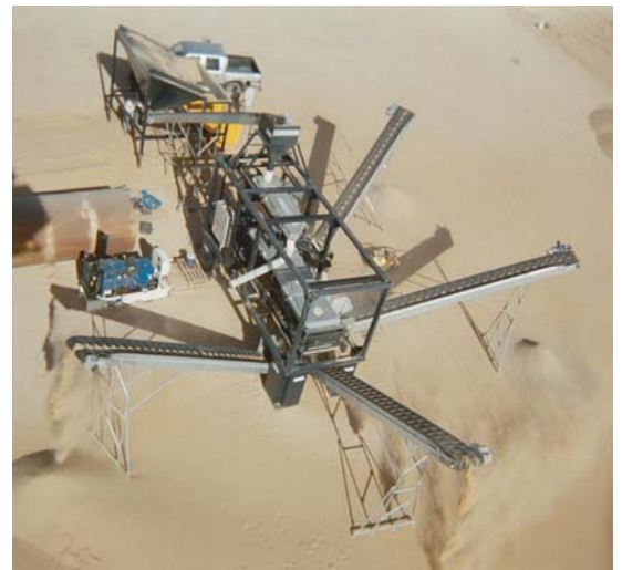
Containerised Sand Grading Plant - specially designed for race course landscaping in Saudi Arabia
