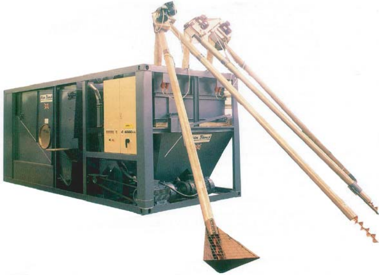
Containerised Feed Mill - 5 tonnes/hour Krasnodar, Russia
