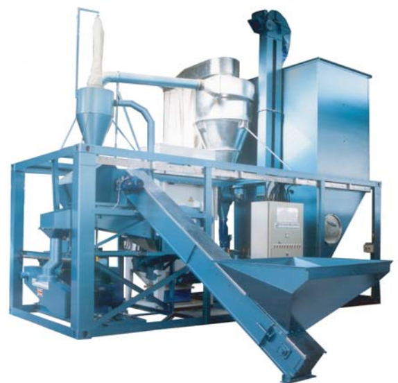
Containerised Milling & Sifting System - specially designed for producing graded pyrethrum (a natural insecticide from crysanthum flowers), Uganda
