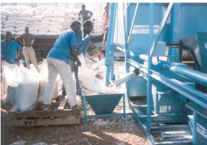
Skid mounted Maize Milling Plant - 8 tonnes/hour - for World Food Programme, Tanzania
