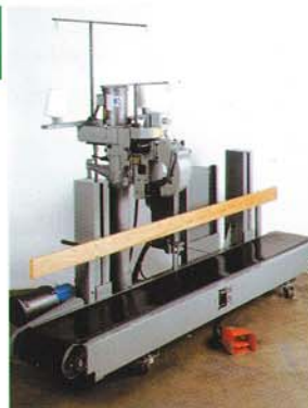
Model MTS: fully automatic stitcher complete with sack conveyor.
